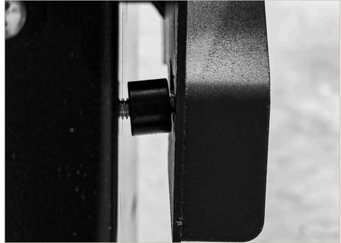
Spacer + bolt, by the drain
