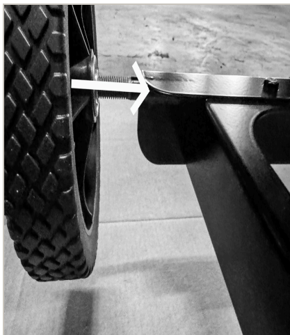
Slide each wheel onto the axle
