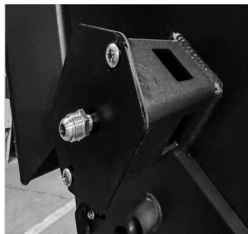
Plate bolts to the burner intake
